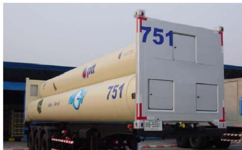
Figure 2.14 - Photo of storage pipes for compressed air (0-3,000psi)
