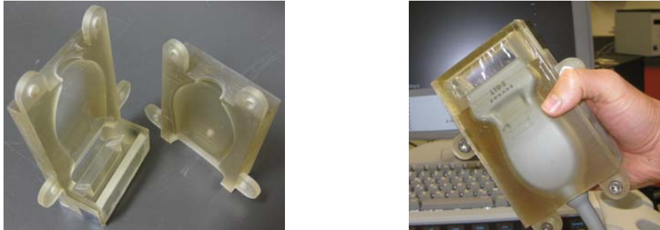
Figure 4. (Left) Two halves of the PED are shown unattached to a clinical probe. A microscope slide serves as the acoustic reflector inside the optical chamber. (Right) The PED mounted to a 10 MHz clinical scanner (Zonare Medical Systems). The acoustic window at the face is made out of 3M™ Tegaderm™. Acoustic coupling to tissue can be achieved by applying acoustic coupling gel, similar to a typical PE examination.
