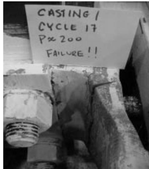
**Figure 12.** Fracture of alpha prototype
