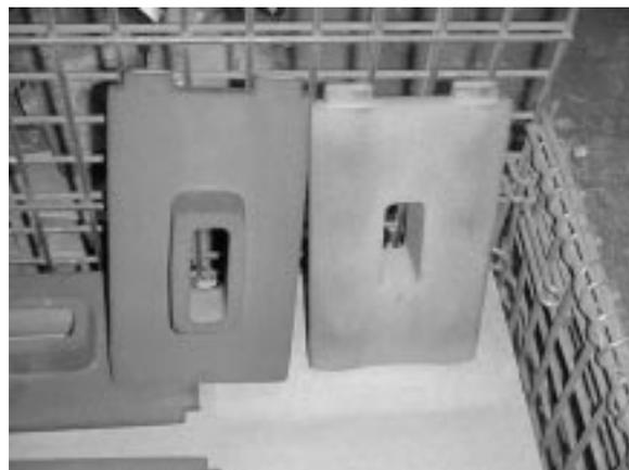
**Figure 10.** Casting Forms for MC: (a) Wood Pattern; (b) Sand Core.
