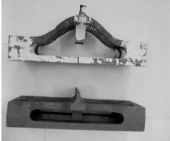
Figure 33. Deformed MC-Base under monotonic loading and undeformed MC-Base
