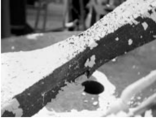
Figure 37. Fracture Plane of MC tested monotonically.
