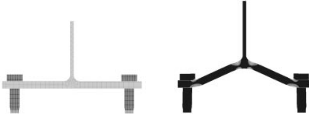
Figure 18. (a) FE model WT 7x49.5 (b) Equivalent plastic strain distribution WT 7x49.5 at 0.067rad
