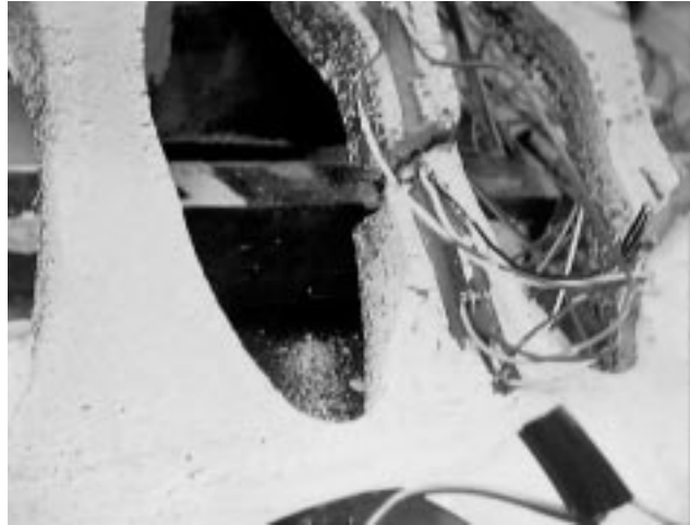
Figure 38. Fracture plane in the middle arm, necking in the outer arms of MC tested cyclically.
