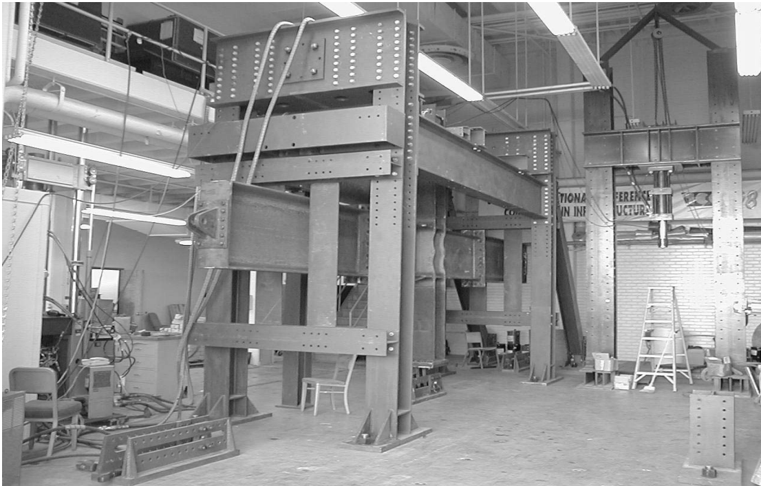
Figure 1. (b): Photo of actual test frame with subassembly prior to test-
