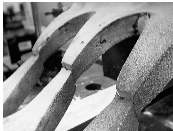
Figure 24. Close up view of the failure region
