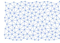
(c) VD-based triangulation for a rectangle-shape sensor net-work.
