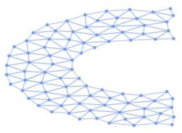
(b) CVT-based triangulation for a *C*-shape sensor network.
