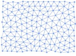
(d) CVT-based triangulation for a rectangle-shape sensor network.
