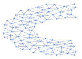
(a) VD-based triangulation for a *C*-shape sensor network.
