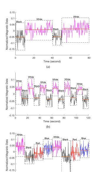
Fig. 1. Magnetometer readings on Y-axis. (a) Change of magnetometer reading due to PC LED display, where the black and magenta waveforms correspond to the black and white images, respectively. (b) Change of magnetic field due to smartphone LED display (black and white). (c) Change of magnetic field while the smartphone sequentially displays white-black-red-blue. The solid orange line in each dashed rectangle box represents the mean of the signal within the box.
