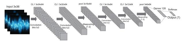
Fig. 3. An example of the proposed deep CNN architectures.
