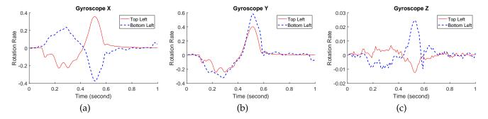
Fig. 6. Comparison of gyroscope data on X, Y, and Z axis while clicking on top-left and bottom-left of the screen.
