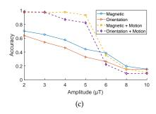
Fig. 8. (a) Noised vs. original magnetic data. (b) E-compass data based on noised and original magnetometer, where the noise is at the level of 8 μT. The resulting error of e-compass reading is only 0.2° in average. (c) MAS accuracy under different noise amplitude.
