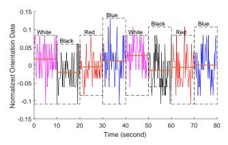
Fig. 5. Change of orientation data while the smartphone sequentially displays four different colors, white-black-red-blue.
