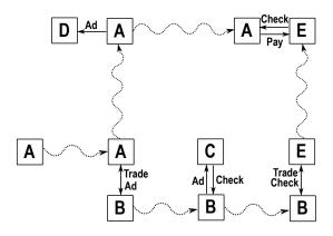
Fig. 1. An example of ad dissemination in a small community where each square represents a node, a dotted curve arrow indicates the movement of a node, and the solid arrow depicts communication. Node A is the ad provider while Nodes C and D are receivers.
