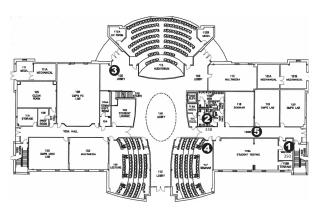
Fig. 4. Placement of RFID readers. Readers 1 and 2 are on the third floor, and Readers 3, 4, and 5 are on the first floor. Reader 1 serves as GR, while other readers are IRs.
