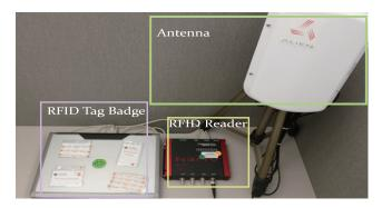
Fig. 5. Our Alien passive RFID gear.
