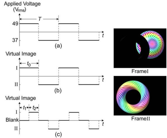
Fig. 2. (Color online) (a) Driving mechanism of the liquid lens, (b) dual-state image rendering mechanism, and (c) tri-state image rendering mechanism for a time-multiplexed dual-focal plane display. The right insets show the image frame I of the occluded sphere on the far focal plane and the image frame II of the torus on the near focal plane.
