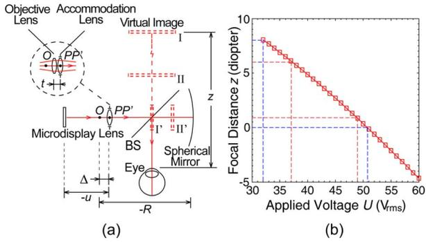
Fig. 1. (Color online) (a) Schematic design of a time-multiplexed dual-focal plane display. (b) Simulation of the focal distance versus the applied voltage of the liquid lens.
