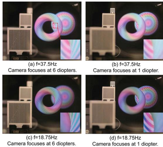
Fig. 3. (Color online) Photographs of the dual-focal plane display (a), (b) with the speed of  $f=37.5$  Hz (Media 1) and (c), (d) of  $f=18.75$  Hz (Media 2). The camera was focused at 6 diopters in (a) and (c), and at 1 diopter in (b) and (d). Insets, zoomed-in images at the boundary of the front torus and back sphere.
