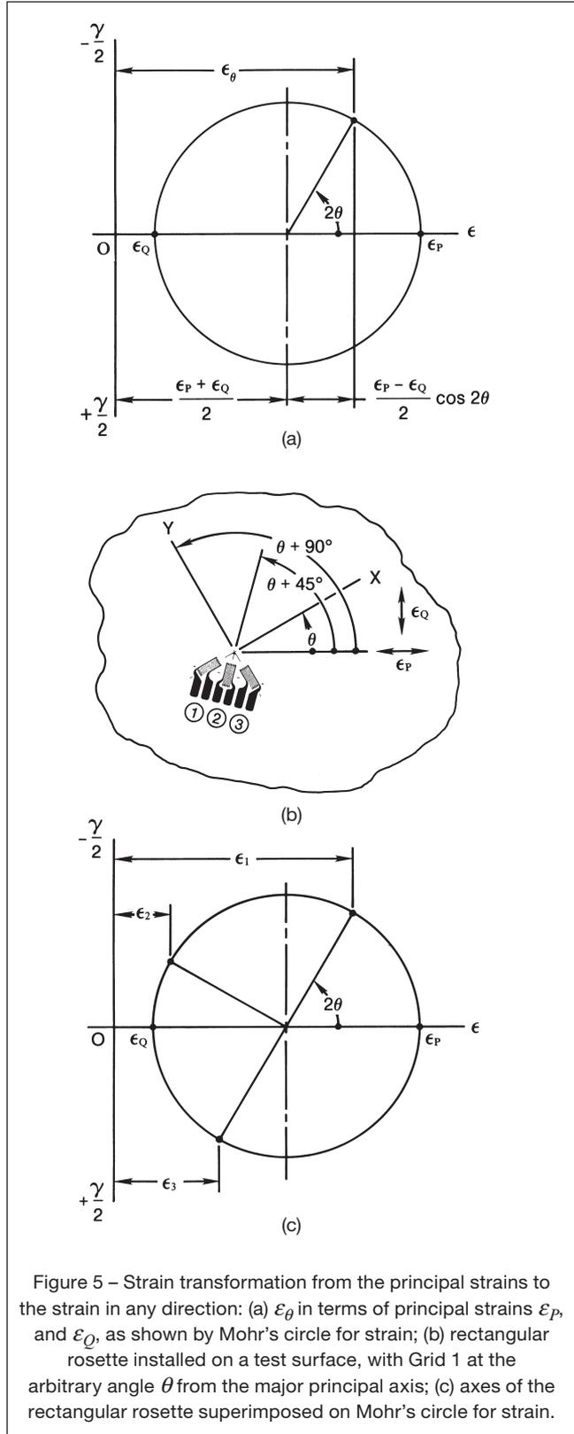
Figure 5 – Strain transformation from the principal strains to the strain in any direction: (a)  $\epsilon_{\theta}$  in terms of principal strains  $\epsilon_P$  and  $\epsilon_Q$ , as shown by Mohr’s circle for strain; (b) rectangular rosette installed on a test surface, with Grid 1 at the arbitrary angle  $\theta$  from the major principal axis; (c) axes of the rectangular rosette superimposed on Mohr’s circle for strain.
