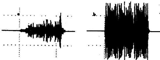
Figure 8. CRT display of digitized waveforms for (a) natural male /s/ (from "stay") used in the "say"-"stay" continua for Experiments 1 and 2, and (b) amplitude-reshaped "hiss" used in the sine-wave continua for Experiment 3.
