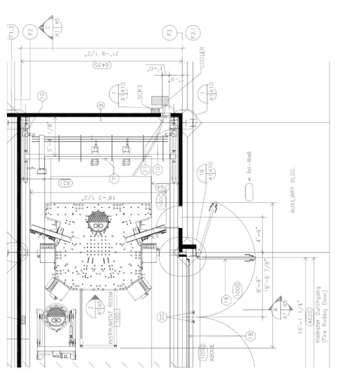
will be used for the clean room tent and LUCIFER maintenance. The LN Stirling cooler is accessible via a hole in the right wall.
