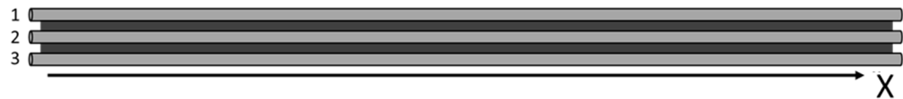
Figure 3. Schematic of the metamaterial composed of a parallel array of three coupled waveguides.
