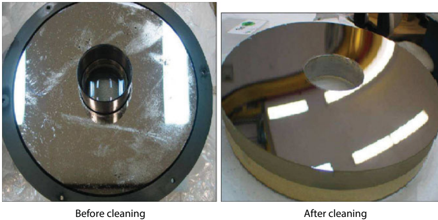
Figure 11.1 A protected aluminum mirror before and after cleaning with Opticlean®. Courtesy of Photonic Cleaning Technologies, Platteville, WI.
