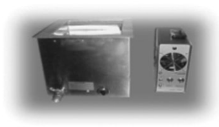
Figure 5.9 Ultrasonic Tank and Generator.
