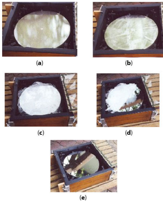
Figure 11.6 Cleaning a small mirror with collodion. (a) Visibly contaminated mirror. (b) The mirror is coated with collodion. (c) Cheesecloth is placed on the mirror to hold the collodion film together when it is peeled. (d) The edges of the collodion film lift up when the film is dry. (e) The cheesecloth and collodion coating are peeled off, leaving a clean mirror surface [72].
