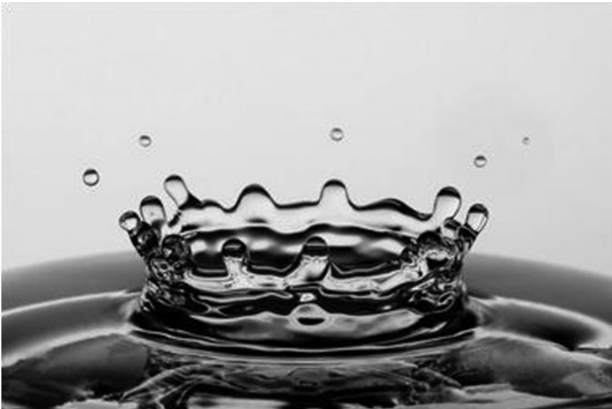
Figure 8.3 Crown formation from droplet impacting a liquid surface.
